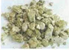
Zonolite Attic Insulation ("ZAI")
